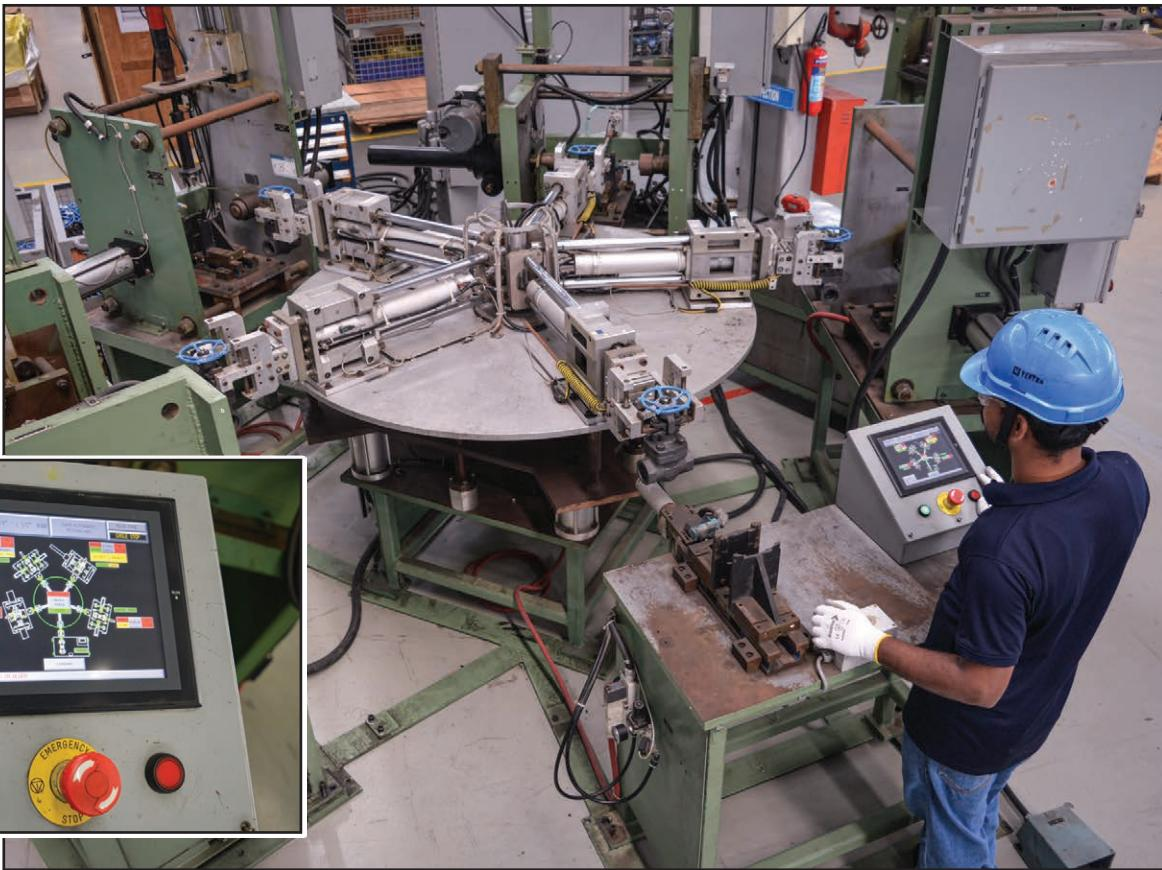
Photos illustrate packing machine and bonnet assembly machine.
