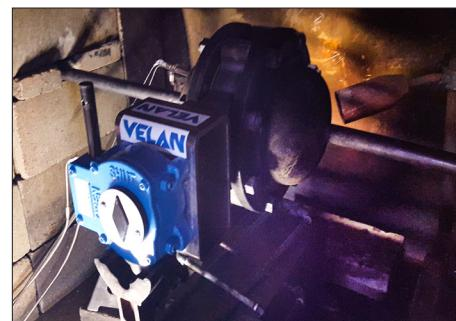
Shock cooled TOV 2.0 after the second fire test.
