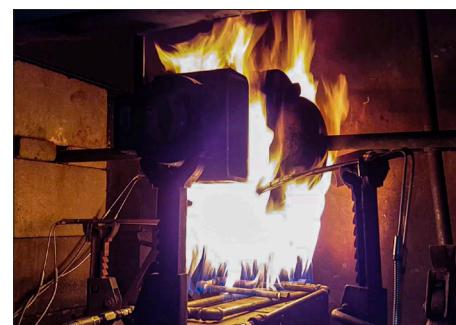
Torqseal® 2.0 triple offset valve at 1650°F (900°C).
