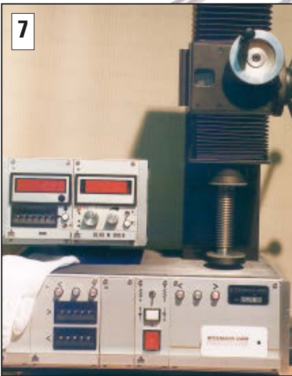
7 Spring rate test verifies force needed to compress bellows.
