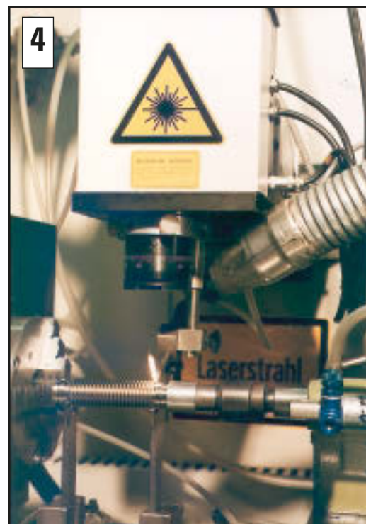
Laser welding of bellows to end rings.
